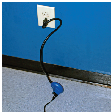
Load Tester plugged in-line with the device
